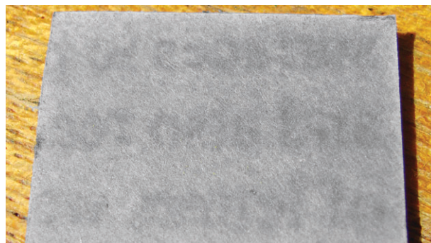
Fig. 3 Close-up of the image obtained when a sample area ( ca. 1” width) from the inside of an envelope, which had been in contact with 12-point inkjet text, was exposed to \text{S}_2\text{N}_2 . Note that before exposure the area appeared completely blank and that the above is the raw image, with no processing to the original digital photograph, save colour removal from the paper. Of course this is a mirror image of the original text; subsequent digital processing can correct this, and further resolve the text via simple contrast enhancement.
